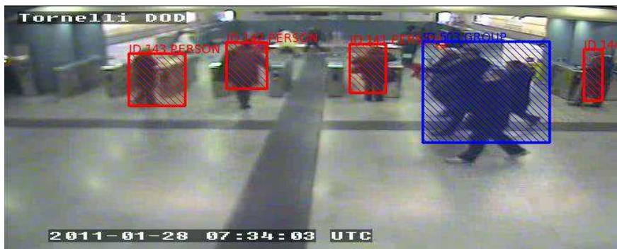
**Figure 10: Example of Ground Truth annotation provided by UNIVIE.**
