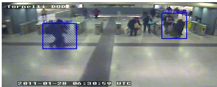
**Figure 16: Illustration of a False Negative (Ground Truth group with ID 101 is not detected), and a False Positive (group with ID 172 is detected but not annotated).**
