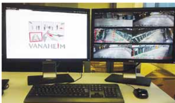
Far right: Fig 2. Passenger flow monitoring at an escalator records and counts each person crossing a virtual boundary.
